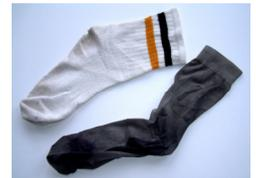
Regarding the test itself, the socks were first analyzed for their nanosilver content. Three of the six socks contained silver particles in the 100-500 nm range; only one contained silver particles in the traditional nanoscale range (under 100 nm). The socks were then washed three times in ultra-pure distilled laboratory water for 24-hour or 1-hour periods using an orbital shaker/agitator. No soaps or detergents were used. The researchers analyzed the resulting washwater.
