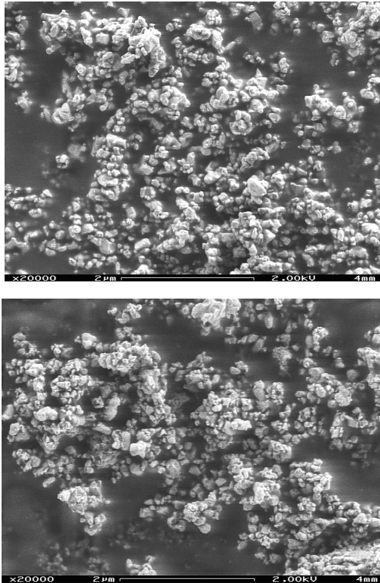
**Figure 1.** Scanning electron micrograph of WC nanoparticles (top image) and WC-Co nanoparticles with 10 wt.% cobalt (bottom image) after preparation with a ball-mill and drying of the particles on the SEM-slide.
