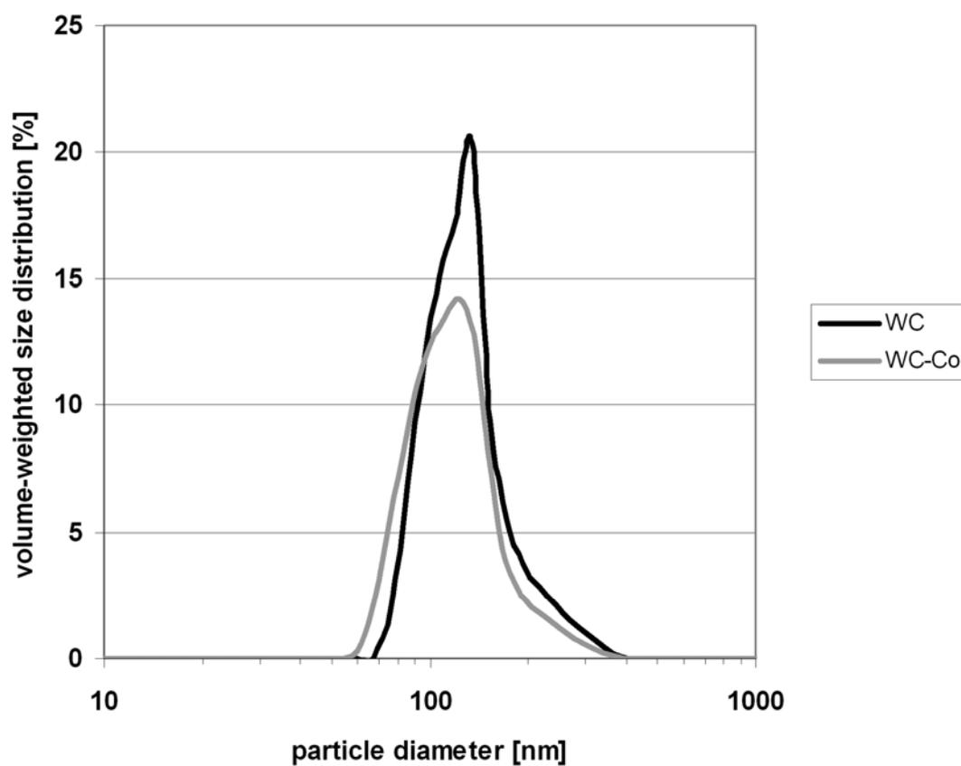
**Figure 2.** Volume-weighted particle size distribution calculated from dynamic light scattering (DLS) data. Based on volume-weighted particle size distribution, a particle size range of 50 to 300 nm was calculated.
