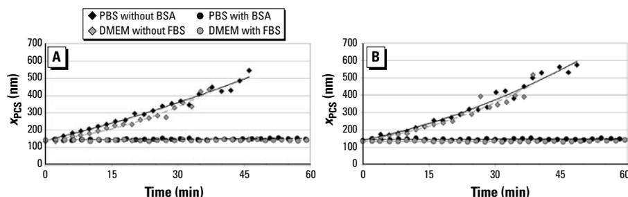
**Figure 1.** Effect of BSA in PBS and 5% (vol/vol) FBS in DMEM on the stability of the WC (A) and WC-Co (B) particles (10 µg/mL) compared to protein-free PBS and DMEM. We found identical results for WC and WC-Co in HBSS (data not shown).
